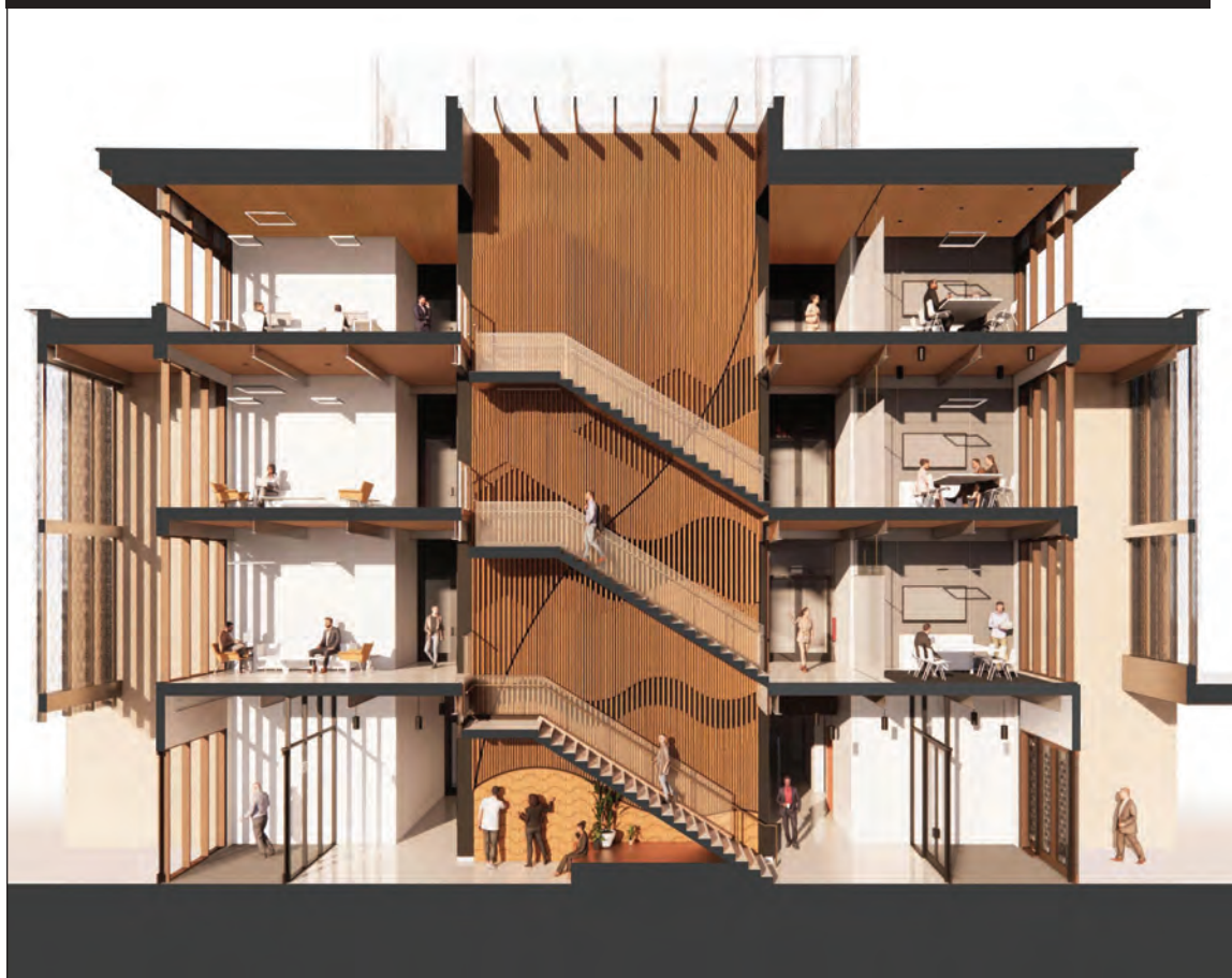
Rendering of the Newhouse mixing chamber featuring a four-story art wall constructed of salvaged timber.
